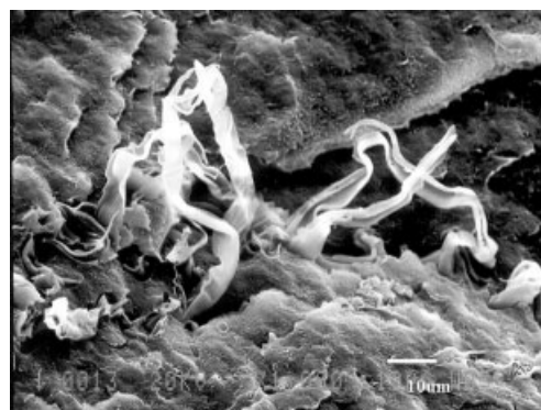
Figure 4 SEM photograph of 1 wt % PBT/PE under condition 2.
